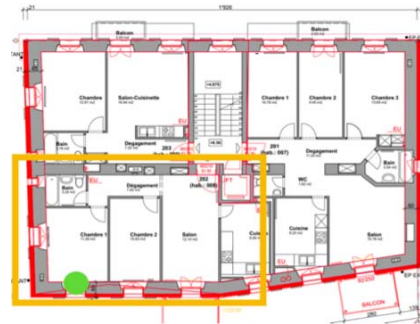
Figure 11: Localisation of the flat at each level (yellow rectangle) and air inlets (green dot)
